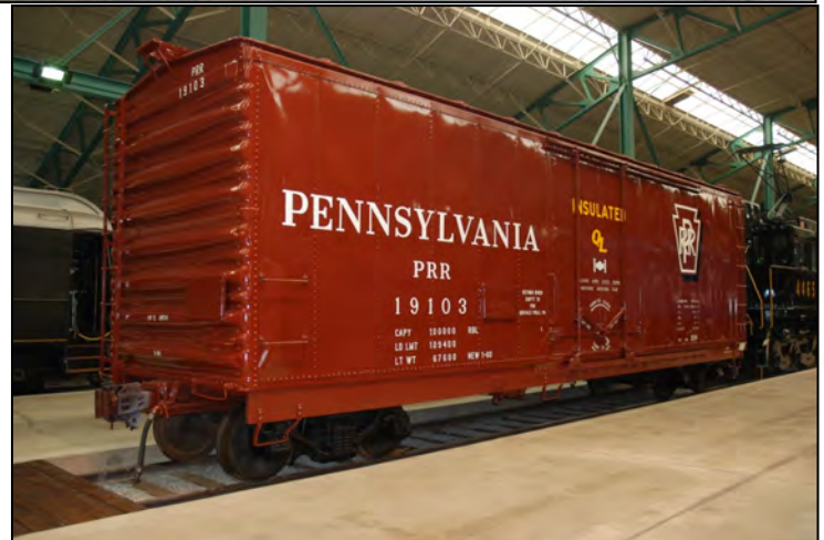
Early 1960s PRR insulated boxcar for Campbell’s soup traffic out of Camden, NJ. Philip Bisatt
