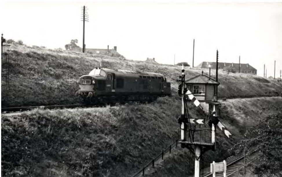
Brand new D6840 running light engine to South Wales passing Patchway Tunnel Box. Note the splitting distant signals. 3rd September 1963 John Sparkes
