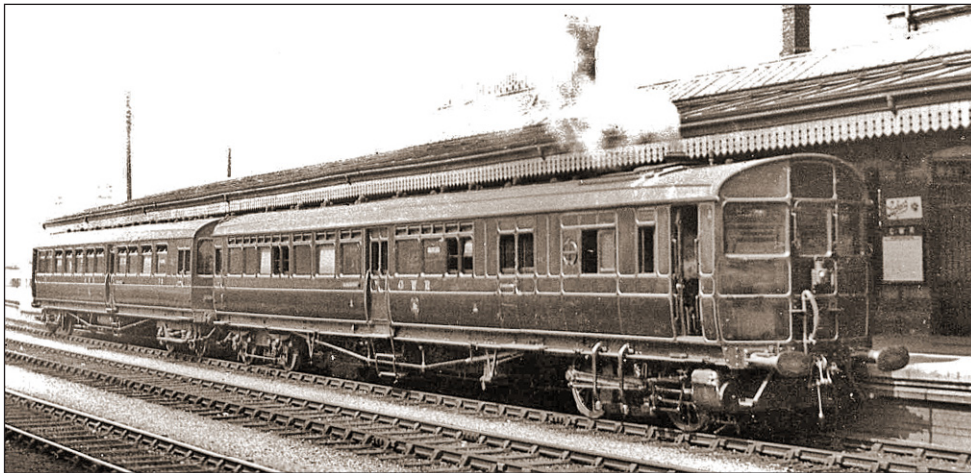
A GWR railmotor and trailer combination, photographed before World War I. These vehicles are almost identical to those being restored by the Great Western Society.
