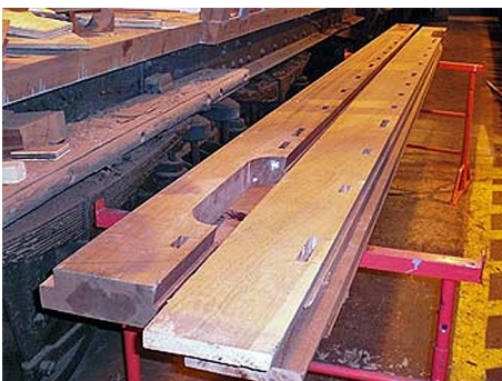
Some of the new bottom rail machined to fit the trailing end of Railmotor No 93.
