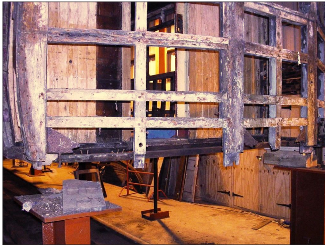
A general view of the trailing end of No 93 in January showing the rotted bottom rail removed, and also the surprisingly good condition of the remaining 100-year-old framework framework.
