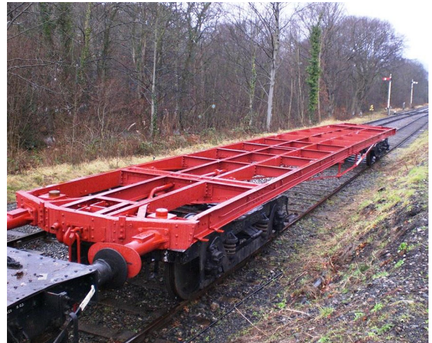
By mid-January the frames of No 93 had been run out from beneath the vehicle body, shot blasted and painted prior to work starting on the retro-conversion to accommodate the newly-built power bogie.
